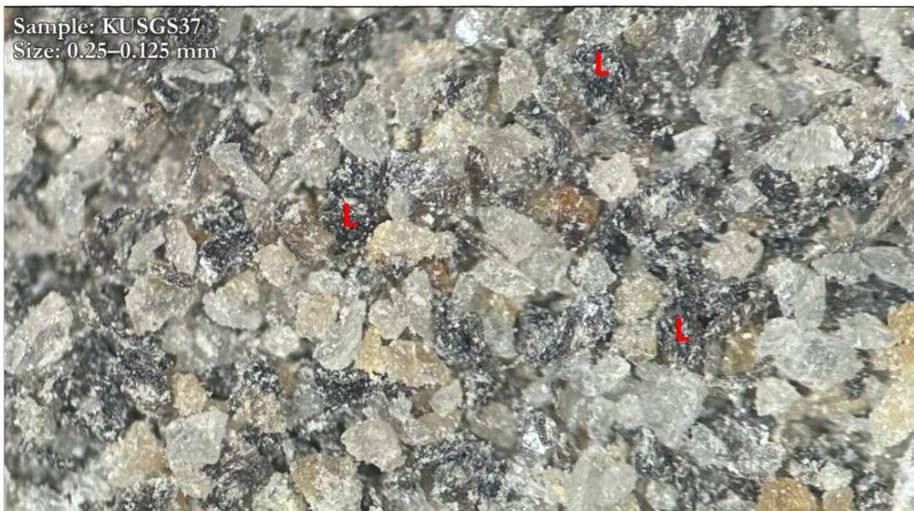
KUSGS37 0.125-0.25mm fine fraction close up. Nearly all black lithium mica crystals are fully liberated in this fraction (Source: [www.greatnorthernminerals.com.au](http://www.greatnorthernminerals.com.au))
