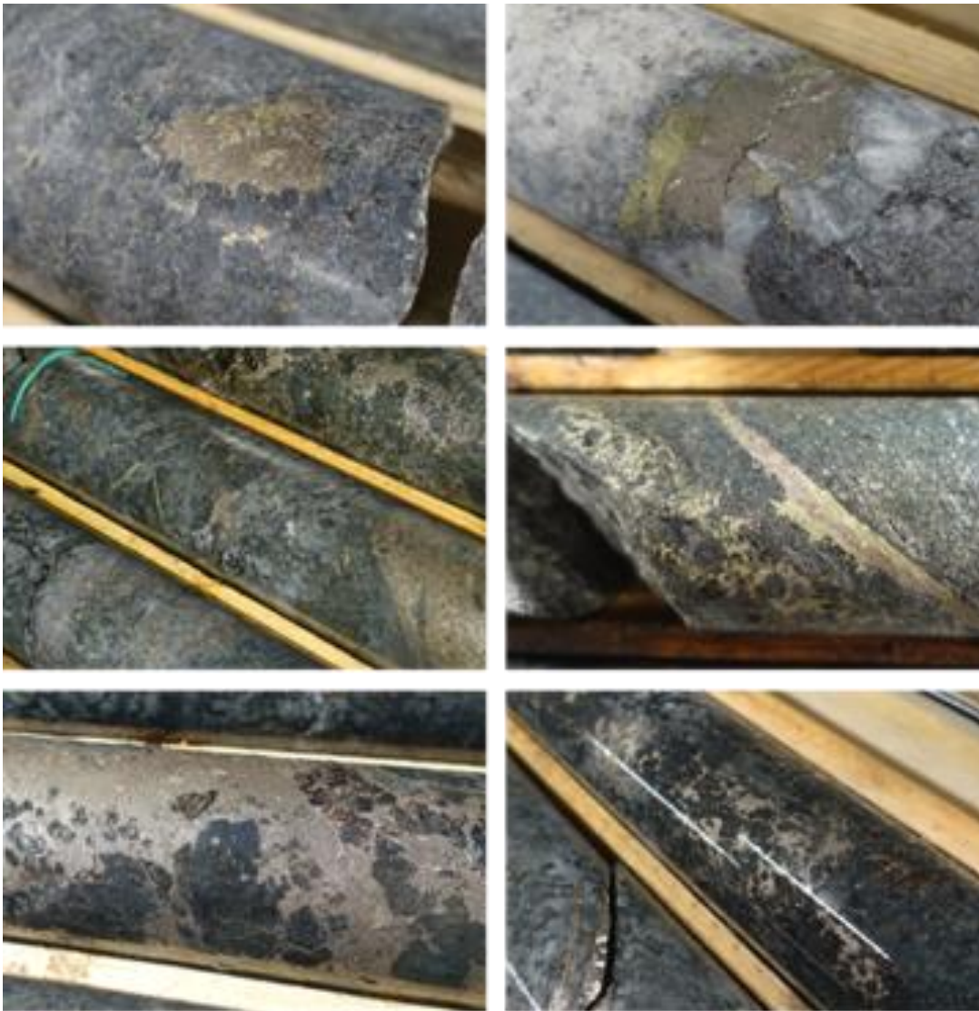
Different magmatic sulfide textures from drilling at Stendalen (Source: www.amaroqminerals.com )
