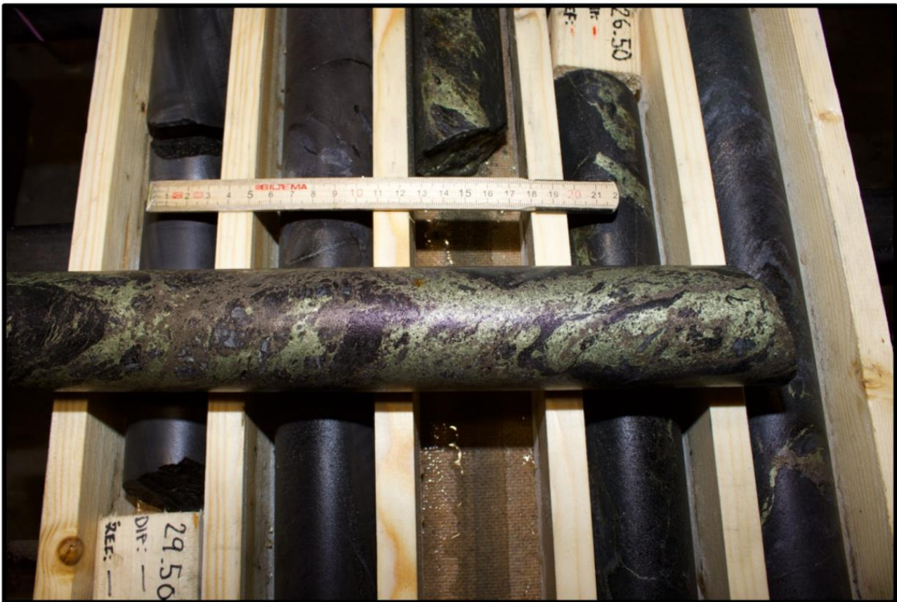
Close-up of the high-grade intersection in drill hole LIL005 (Source: www.plethora-exploration.com )
